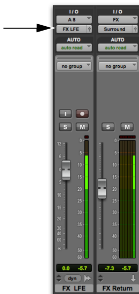
Discrete LFE routing, with main output to mono LFE channel
