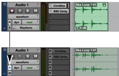
Frozen audio track, before and after—Freeze icon highlighted
