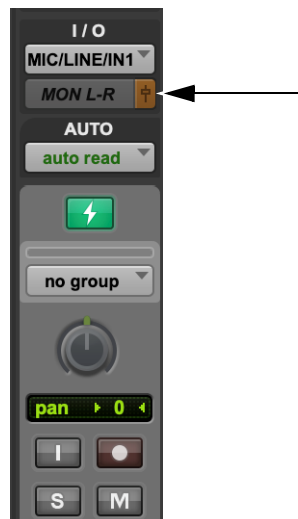
DSP Mode-enabled, track output inactive due to insufficient resources
