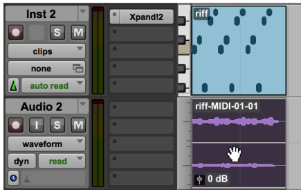
Audio rendered by dragging and dropping a MIDI clip from an Instrument Track (top) to an audio (bottom)
