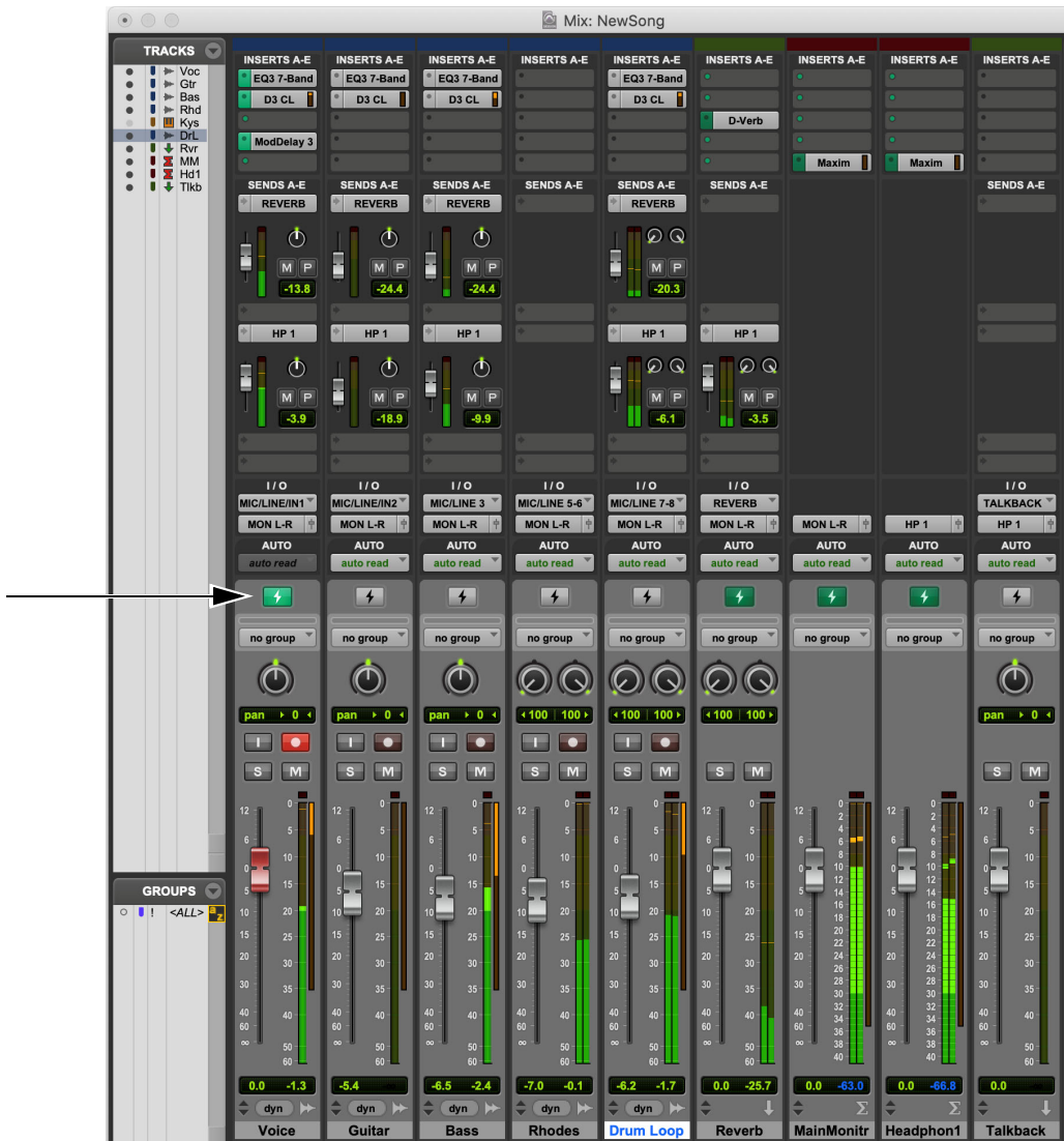
Figure 4. Recording vocals in DSP Mode for ultra-low latency monitoring
