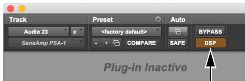
DSP Mode, DSP plug-in inactive due to insufficient DSP resources
