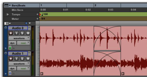
Two adjacent multitrack clip groups with crossfades on the audio tracks, but not on the MIDI track
