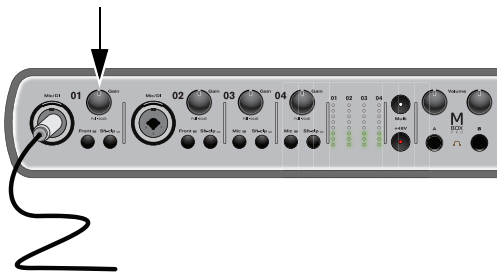
Input 1 Gain on Mbox Pro
