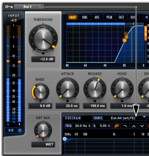
Configuring a key input for side-chain processing
