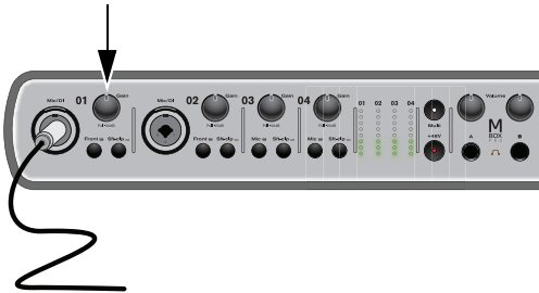
Input 1 Gain on Mbox Pro
